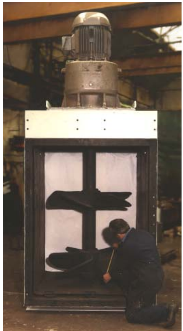
'1300' Floatex Attrition Scrubber showing the rubber covered impellers and optional wear plates.
