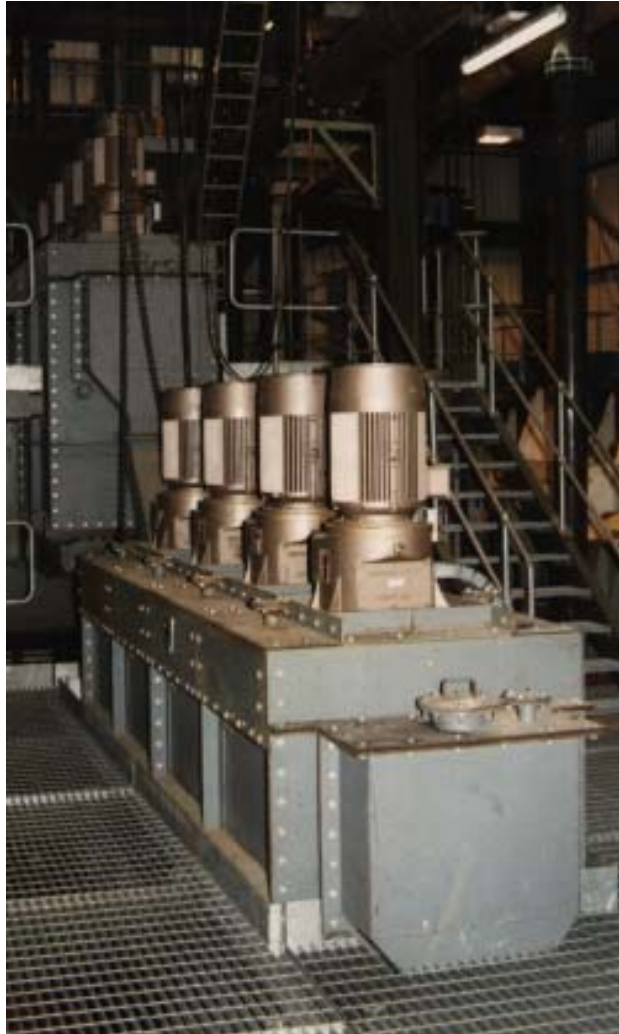
4 Cell '1000' Floatex Attrition Scrubber with optional covers for gas purging
